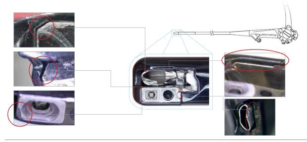
References for cracking (38) and holes (39): Crack / Scratch / Hole
